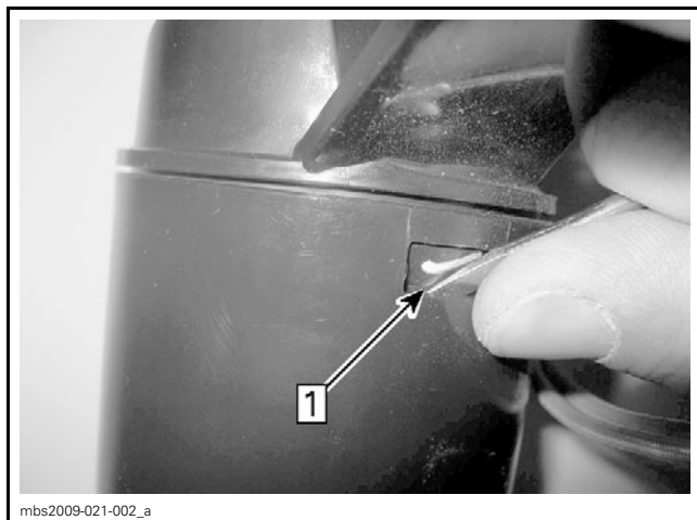
Step 1: Insert screwdriver between tab and sump tank
