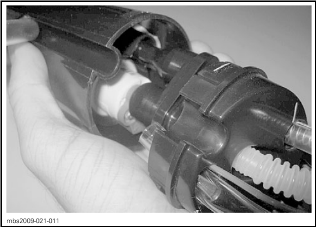
STEEL MESH FILTER, FUEL PUMP REMOTE PICK-UP
