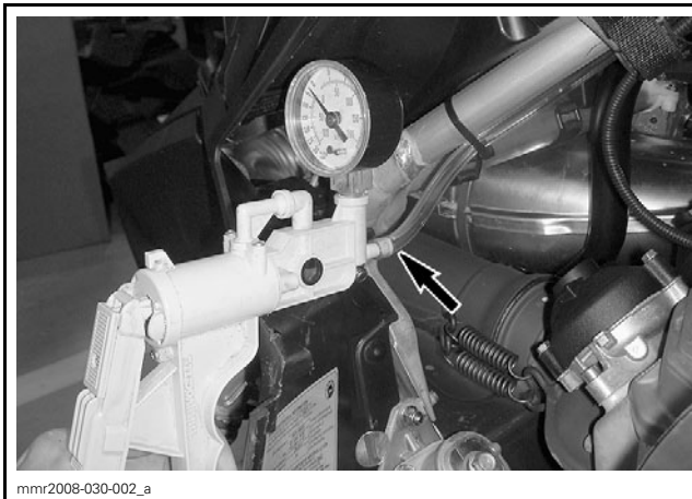
TYPICAL - VACUUM/PRESSURE PUMP ON VENT TUBE
