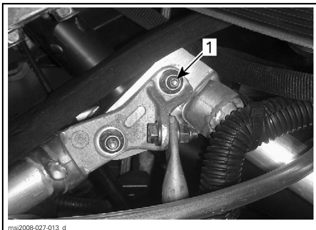
1. Mounting bolt, front frame member
