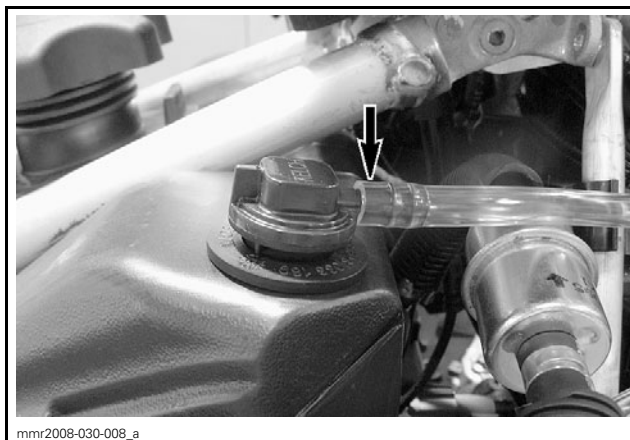
TYPICAL - DISCONNECT FUEL VENT TUBE
